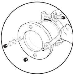
Move the Dismantling Joint into position between the mating flanges. Remove the outer nuts of the tie-rods on both sides and insert the rods into holes in one flange.
