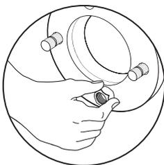
Replace the outer nuts on the other side of the flange.
