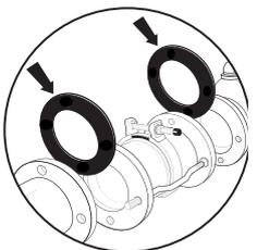
Insert the proper-sized flange gaskets (not provided) between the flange faces on both sides.
