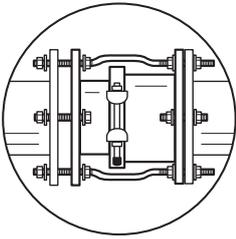
Expand the Dismantling Joint until both flanges are flush. Attach the Dismantling Joint to the opposite mating flange in your system and fasten together with flange bolts.
