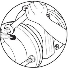
Tighten the INNER nuts against the flanges on both sides.
