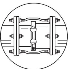
Recharge the line and check for leaks. If any leakage across the seal end is evident, reduce the pressure in the line and increase the labeled torque of the end ring bolts by up to 50%.
