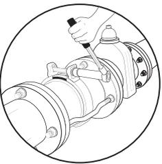
Tighten the bolt on the end ring (in sizes 50-300mm). On sizes 350-600mm, cross-tighten the bolts evenly on each side of the end ring. Tighten the end ring bolts to the right torque as indicated on the label.
