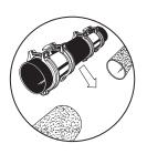
Slide the two HYMAX GRIPs on both sides the replacement pipe. Lower the replacement pipe and the two grips positioned on it into the ditch.
