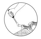
Tighten the end rings using a torque wrench, to the correct torque shown on the product's label. By tightening bolts the couplings are steadily stabbed on the pipe.
