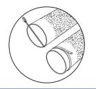
Measure the pipe's outside diameter and make sure the coupling's size fits properly.
