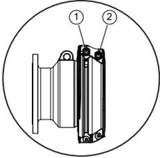
Tighten the end ring using a torque wrench, to the correct torque shown on the product's label.
