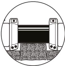
**NOTE:** Make sure that the pipe is properly supported. HYMAX GRIP Flange Adaptor cannot support the weight of the pipe by itself.
