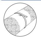
Measure the pipe TWICE using an OD tape. Select the appropriate clamp to fit the outside diameter of the pipe. Unpack it carefully.
