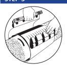
Center the EZ-MAX over the leak or damaged section of pipe till it covers the marks (step 3). Fully rotate the clamp around the pipe by pulling the nut side compression beam over, underneath, and back around the pipe.
