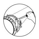
Tightening the end rings. Tighten the coupling bolts using a 23.81mm (15/16") socket wrench for 350-600mm couplings, and a 38.10mm (1.5") socket wrench for 650-1500mm couplings. Tighten the bolts evenly on each end ring in an alternating pattern to the torque mentioned on the label. Cross-tightening ensures that the gasket is evenly seated. When you finish, re-check the torque again.
