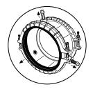
Unscrew the centering pins. Use an open-ended wrench or socket wrench to retract the centering pins. This allows the coupling to be stabbed over the pipe end without interference, and also allows for proper positioning.
