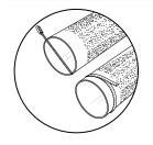
Measure the pipe's outer diameter and make sure the coupling being used has the proper OD range. Always use an OD tape to ensure that you are using the proper size coupling
