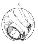
Once the REPAMAX is around the pipe, engage the compression beam until it "clicks" into the 1st closing position (see below). The REPAMAX can now be positioned over the leak covering the marks on both sides (see step 4).
