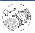
Set the centering pins. Secure the centering pins using an open- ended wrench or a socket wrench. Make sure the "o" ring on each centering pin seats properly beneath the pin head. Fully tighten the centering pins into the coupling body. The pins prevent the coupling from drifting along the pipe. They are not "set screws".
