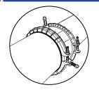
Positioning the Reducer for installation. If possible, place the Reducer(s) on the replacement pipe (on both ends) and lower the pipe and couplings into the ditch. Slide the couplings outward so that they cover the minimum marks made in Step (4).
