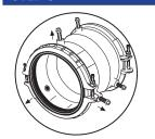
Unscrew the centering pins. Use an open-ended wrench or socket wrench to retract the centering pins. This allows the Reducer to be stabbed over the pipe end without interference, and also allows for proper positioning.
