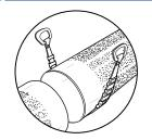
Prepare the pipe ends. Clean and de-scale each pipe end. Remove any debris or build up on the pipe ends. Clean the outer pipe surface with water. Clean each pipe end to a length of the coupling body.
