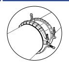
Positioning the Coupling for installation. If possible, place the coupling(s) on the replacement pipe (on both ends) and lower the pipe and couplings into the ditch. Slide the couplings outward so that they cover the minimum marks made in Step (4).
