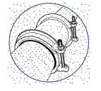
Position the coupling for installation. If possible place the coupling(s) on the replacement pipe (on both ends) with top-facing bolts and lower the pipe and couplings into the ditch. Slide the couplings outward so that it covers the marks made in step 4.
