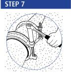
Tighten the end rings. Tighten the coupling bolts to the right torque shown on the product's label. When you finish, re-check the torque again.
