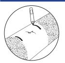
Mark the pipe an even distance from the break or leak according to the length of the EZ-MAX.
