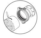
Mark pipe end to a minimum required stab depth. This mark indicates the required stab depth for the HYMAX GRIP Flange Adaptor.
