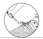
Tighten the end ring using a torque wrench, to the correct torque shown on the product's label.
