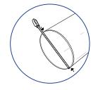
Measure both pipes' outer diameters and make sure the Reducer's size will fit the pipes properly on both sides which are different in diameter.
