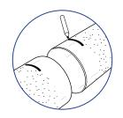
Mark each pipe end to a minimum required stab depth. This mark indicates the required stab depth for the HYMAX Reducer.
