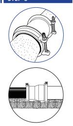
Position the coupling for installation. Make sure that the different product diameters fit the different pipes. Place the coupling on the pipe with top-facing bolts. Slide the coupling so that it covers the marks made in step 4. Make sure that the pipes are not touching inside the body of the HYMAX. There must be space between the pipes in order for continuous dynamic deflection (CDD) to take place. Make sure that the pipes are properly supported.
