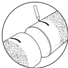
Mark each pipe end to a minimum required stab depth. This mark indicates the required stab depth for the coupling.
