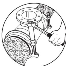
Tightening the end rings. Tighten the coupling's bolts using a 19.05mm (3/4") socket wrench for 40-80mm couplings, a 22.23mm (7/8") socket wrench for 100-300mm couplings, a 23.81mm (15/16") socket wrench for 350-600mm couplings, and a 38.10mm (1.5") socket wrench for 650-1500mm couplings. Tighten the bolts evenly on each end ring in an alternating pattern to the torque mentioned on the label. Cross-tightening ensures that the gasket is evenly seated. When you finish, re-check the torque again.
