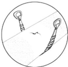
Prepare both pipe ends of the existing pipe by descaling if required. Clean the pipe as required using water. Make sure that the pipes are clear from debris and defects that may interfere with the HYMAX Outlet's proper seal.
