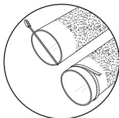
Measure the pipes' OD twice and make sure the coupling's size will fit the pipes properly.
