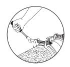
Tighten the end rings using a torque wrench, to the correct torque shown on the product's label. By tightening bolts, the reducers are steadily stabbed on the pipe.
