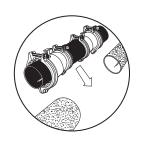
Position the reducer for installation. Make sure that the different product diameters fit the different pipes. Now slide the reducer on both sides of the replacement pipe. Lower the replacement pipe, and the two reducers positioned on it, into the ditch.
