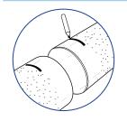
Mark each pipe end to a minimum required stab depth. This mark indicates the required stab depth for the coupling.
