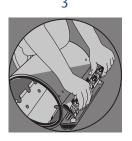
Once the REPAMAX is around the pipe, engage the compression beam until it "clicks" into the 1st closing position. The REPAMAX can now be positioned over the leak covering the marks on both sides (see step 5).
