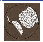
Mark each pipe end to a minimum required stab depth. This mark indicates the required stab depth for the HYMAX Flange Adaptor.
