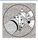
Tightening the end rings. Tighten the Flange Adaptor's bolts using a 22.23mm (7/8") socket wrench for 40mm-80mm couplings, a 22.23mm (7/8") socket wrench for 100mm-300mm couplings. When you finish, re-check the torgue again.
