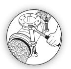
**NOTE:** Use of a torque wrench to tighten the bolts is required. A torque wrench will assure a proper torque has been applied to the coupling. Do not use other tools to tighten the coupling's bolts!
