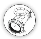
Unpack the coupling. Carefully remove the coupling from its packaging. Inspect the coupling, if the end rings are not centered on the coupling DO-NOT-USE. Contact your distributor for return and replacement! DO NOT attempt to hammer the end ring into place! This will damage the end ring and void the warranty!
