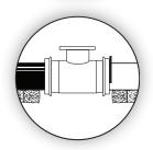
**NOTE:** HYMAX is not designed to support the weight of the pipes by itself. For uncoated ductile iron, grey cast iron and asbestos cement pipe surfaces appropriate water-based gasket lubricant is required on both gaskets inside surface and pipe's outer surface.
