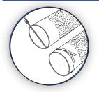
Measure the pipes' OD twice and make sure the coupling's size will fit the pipes properly.
