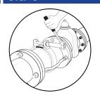
Tighten the bolt on the end ring (in sizes 80-280mm). On sizes 300-600mm, cross-tighten the bolts evenly on each side of the end ring. Tighten the end ring bolts to the right torque as indicated on the label.
