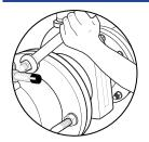
Insert additional bolts and nuts through the remaining holes in the flanges to tighten the Dismantling Joint to both flanged products. Tighten the INNER nuts against the flanges on both sides.
