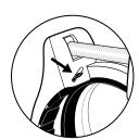
For final placement insert the protrusion into its intended slot – see drawing - and press hard with your thumbs until the protrusion in the other end sits well in place.
