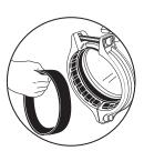
**NOTE:** Do not remove the inner gasket unless the OD falls within the upper range of the product. The proper range sizes are shown on the product label.
