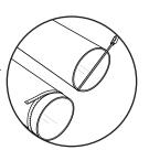
dents, flats or other defects which may interfere with the GRIP SWIVELJOINT's proper seal. The GRIP SWIVELJOINT may not fit well or function properly on pipe which is out of round or damaged.
