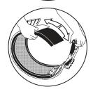
(C) Open up the REPAMAX fully while positioning it over the leak
