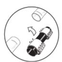
Slide The REPAMAX outward so that they are centered over the area to be joined covering the marks on the pipes.
